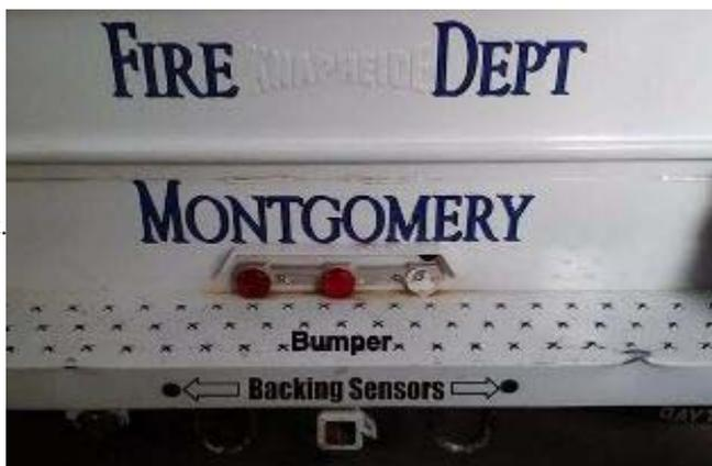
Shown above: Backing Sensors on Montgomery Fire Vehicle
